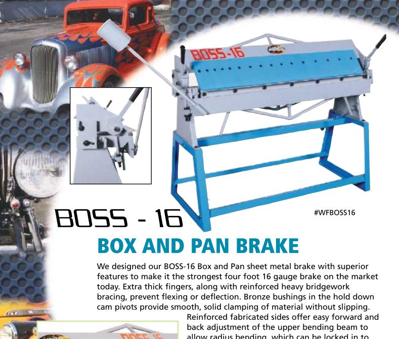
Reinforced fabricated sides offer easy forward and back adjustment of the upper bending beam to allow radius bending, which can be locked in to prevent movement. No more rotating a cam in the back where it can slip. A heavy, adjustable counterweight assembly aids in bending heavier materials. 16 removable fingers in sizes 2", 3" and 4" can quickly be adjusted to accommodate a box size up to 48" width. Deep finger depth allows
